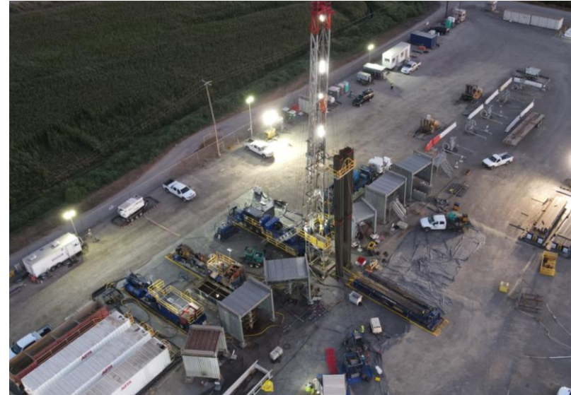
Typical well site with rig performing well inspection. Multiple wells are removed from service due to close spacing layout of facility.
