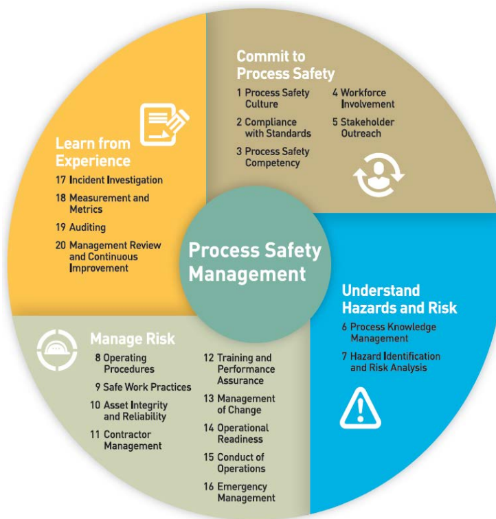
Figure 6 – The PG&E Process Safety Method
