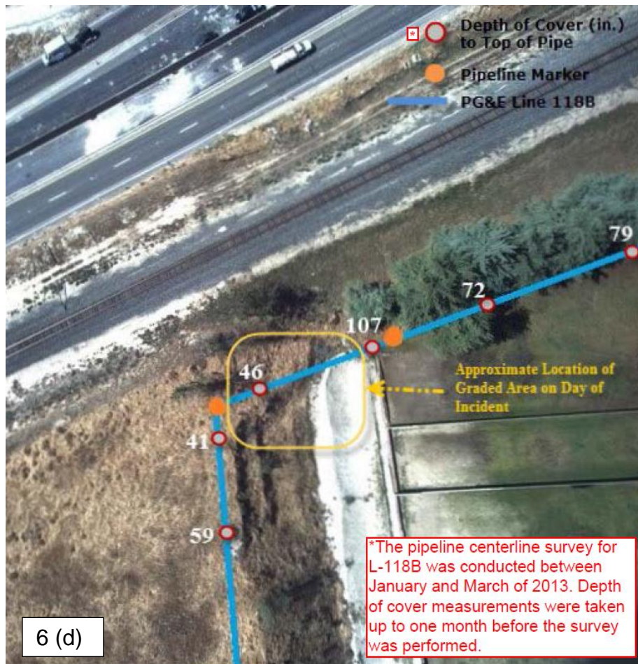
Figure 6 (d): PG&E 2013 centerline survey results
