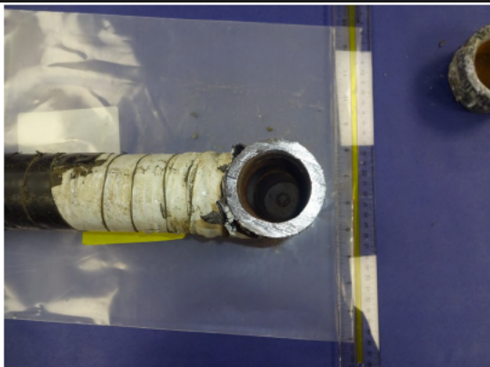
Figure 6. Bottom view of Mueller Tee showing bottom of X-Pando Plug. 3
