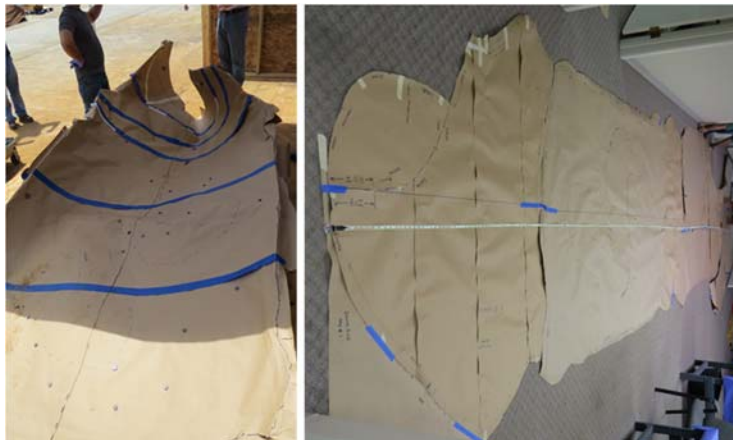
Figure 9: Reconstruction of pipeline failure using paper method
