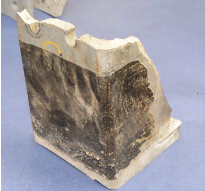
Figure 22. Photograph of the Stub C base fracture during visual examination.
