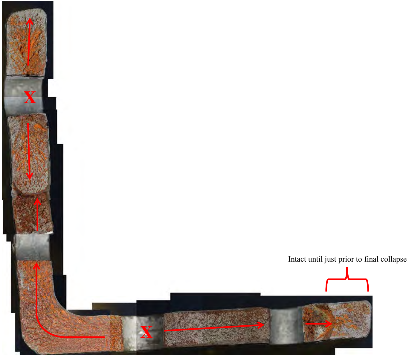
Figure 28. Stub D tower-side fracture surface montage, when viewed from below. “X” indicates the hole at the fracture origin, and red arrows show crack growth directions. The red bracket indicates the area that was intact until just before the final tower collapse.
