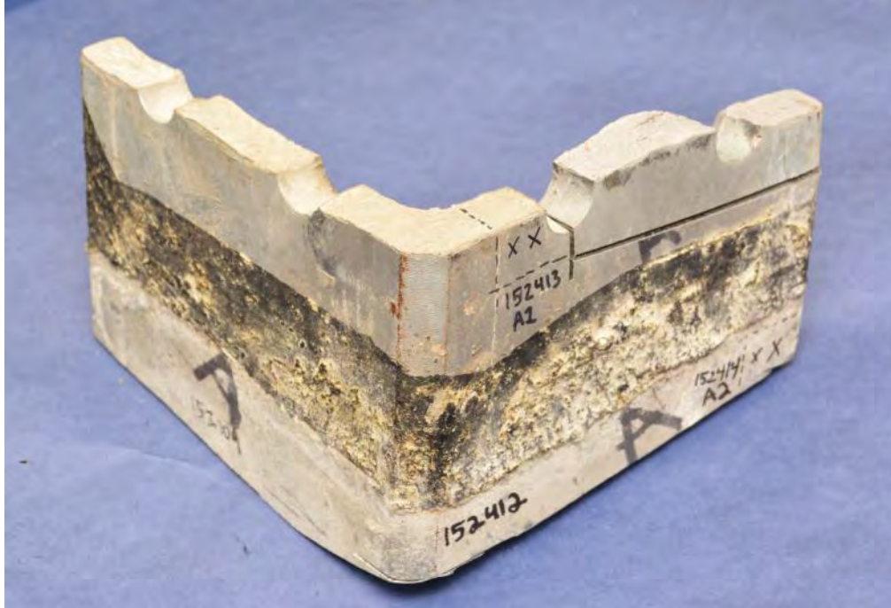
Figure 20. Photograph of the Stub A base fracture during visual examination.
