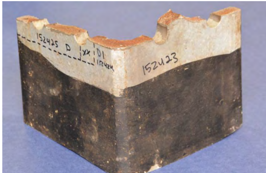
Figure 23. Photograph of the Stub D base fracture during visual examination.
