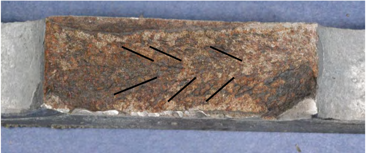
Figure 25. Photograph that shows representative chevron marks in Stub B. The dark lines help show the direction of the chevron marks.
