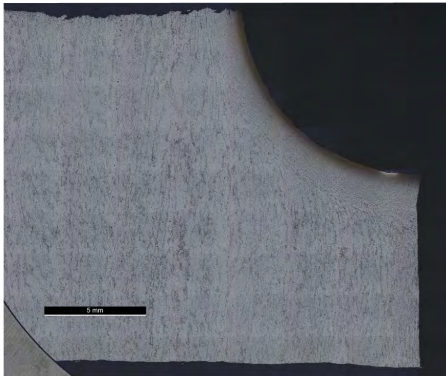
Figure 31. Low-magnification metallographic montage that shows microstructure at and away from one of the two Stub D punched-hole fracture origins.
