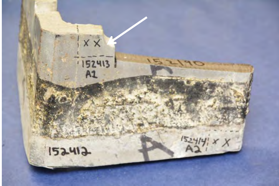
Figure 30. Photograph that shows representative sectioning location for metallographic analysis in Stub A (indicated by arrow). The “x x” indicates the metallographic section location.
