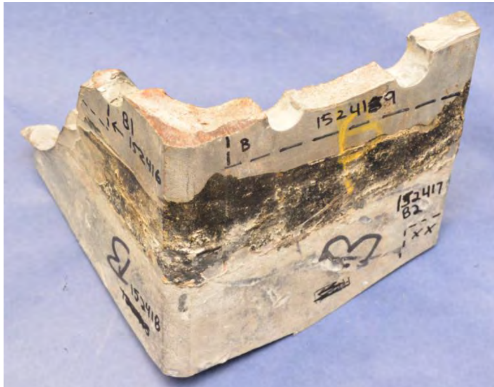
Figure 21. Photograph of the Stub B base fracture during visual examination.
