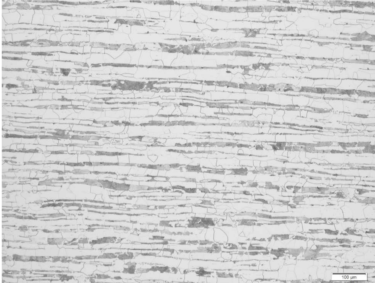
Figure 17. Photomicrograph of Mount M3 showing the microstructure of the pipe body away from the leak and away from the ERW weld. Magnification – 100X. Nital etch.
