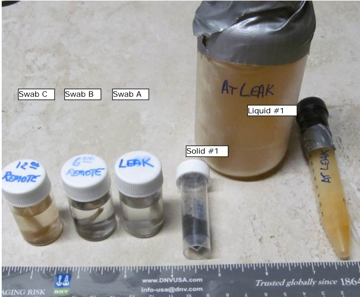
Figure 3. Surface swabs, solid, and liquid samples collected by DNV GL personnel in the field when the pipe section was cut out.
