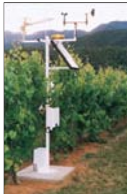
This vitaculture site in Australia integrates meteorological, soil, and crop measurements.
