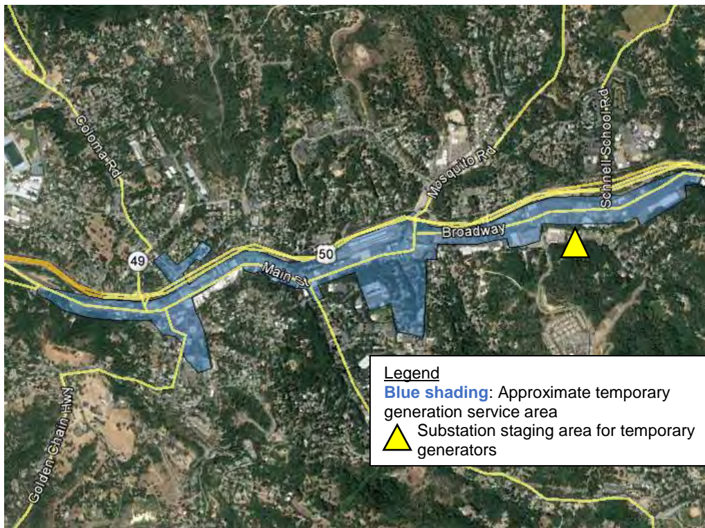
Figure 15: Approximate area served by PG&E Temporary Microgrid in Placerville
