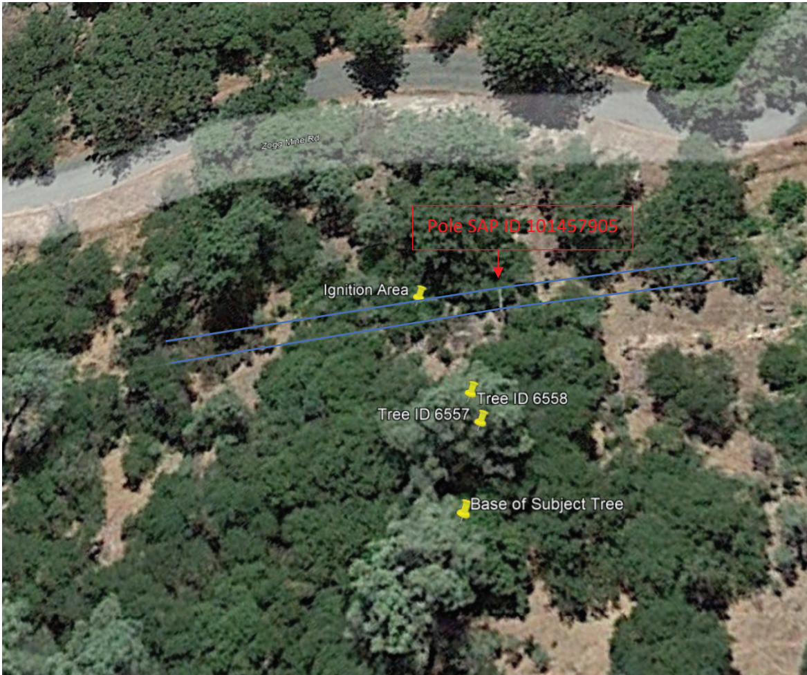
Figure 1: Diagram of the Base of the Subject Tree, Tree ID 6557, Tree ID 6558, Ignition Area, and PG&E Facilities. 25 The lines marked in blue show approximate conductor path and continue east and west in both directions. The pinned locations of Tree IDs 6557 and 6558 are based on GPS coordinates from PG&E VM records. The location of the Subject Tree is based on CalFire's GPS records. All locations represent the approximate locations of the base of the
