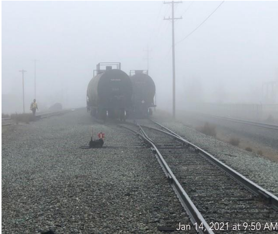
Tank car located on the left side track is fouling the adjacent track
