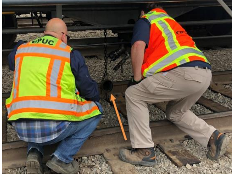
Bottom outlet cap not applied underneath the tank car
