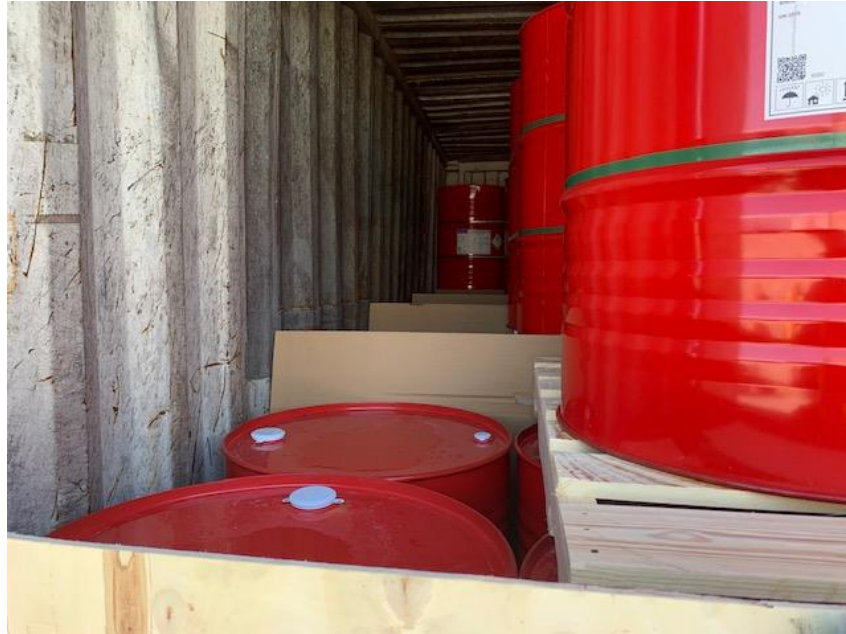
Voids next to steel drums which would allow for loads to shift laterally
