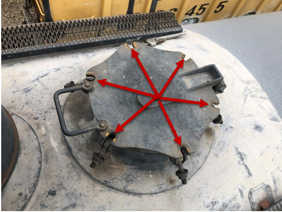
Six manway swing bolts not secured
