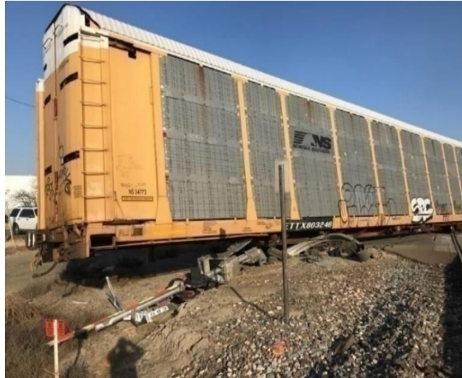
Empty rail car derailed at street crossing
