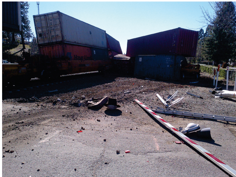
January 2013 derailment, Grass Valley Road at-grade public highway crossing, near Local Safety Hazard Site No.12 in Colfax, CA. Cause was due to equipment failure: tread build up on flange wheel.
