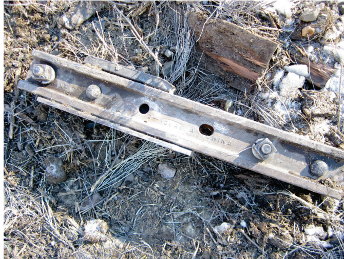
An example of inadequate rail repair which lead to a December 2013 derailment at Local Safety Hazard site No. 16 near Tehachapi CA.
