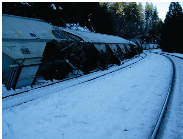
2011 UP derailment at Local Safety Hazard Site No.12, near Gold Run, CA. Cause was due to remote locomotive mechanical failure.
