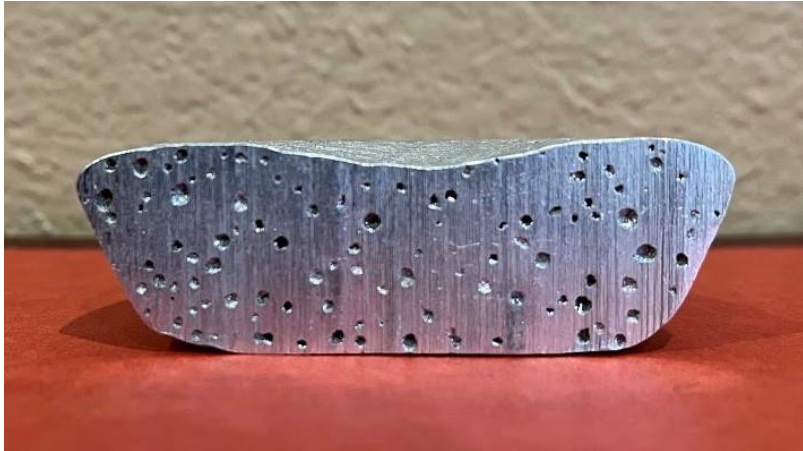
Aluminum with high dissolved hydrogen.
