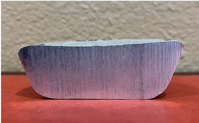
Aluminum with low dissolved hydrogen.
